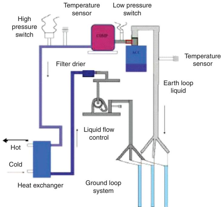
**Figure 2.** Typical application of a borehole heat exchanger (BHE) heat pump system in a central European home
