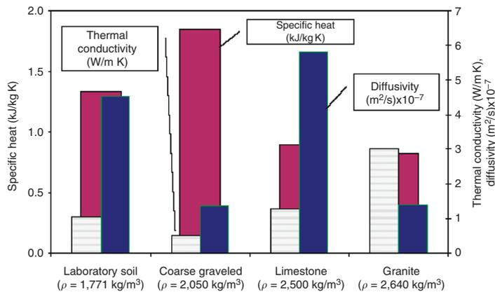
**Figure 1.** Measured thermal properties for different soils
