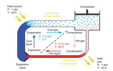
Figure 6. Heat pump works by promoting the evaporation and condensation of a refrigerant
