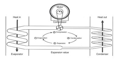
Figure 4. Ground source heat pumps
