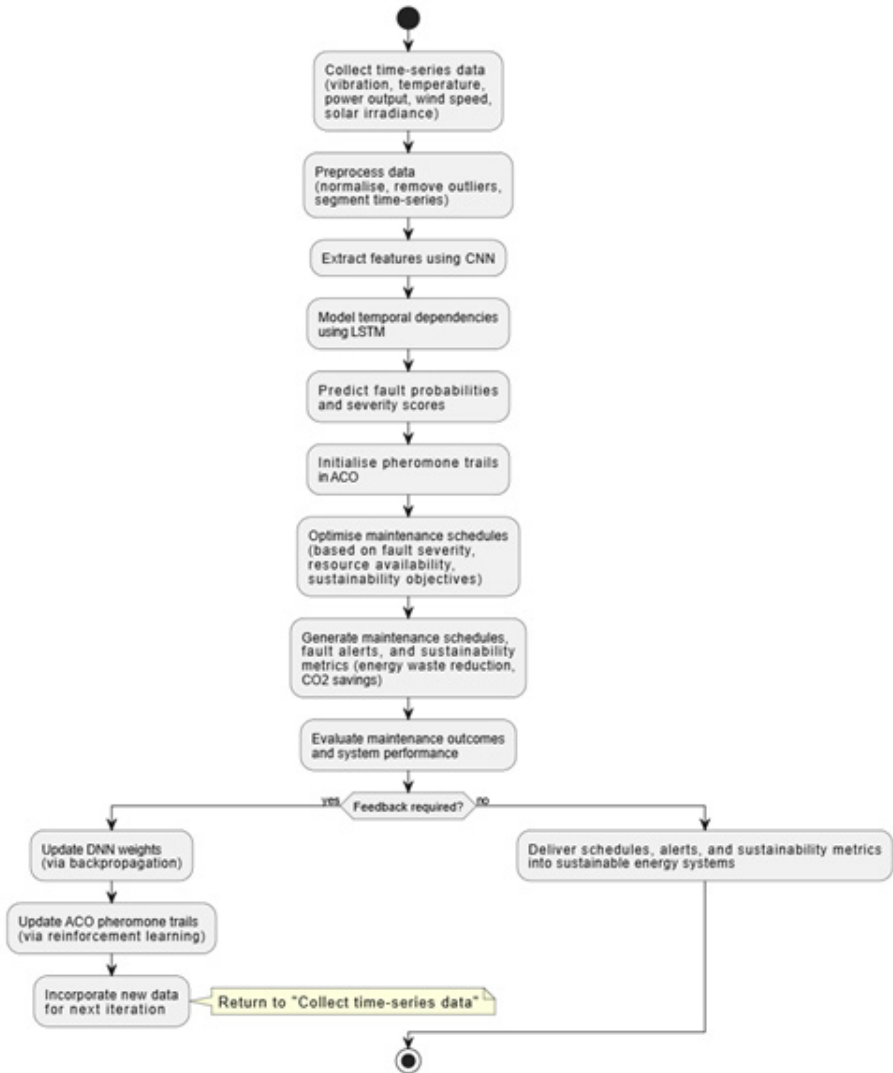
Figure 1: Hybrid CNN-LSTM and ACO Framework for Predictive Maintenance in Sustainable Energy Systems
