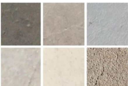
Figure 2 Graphical Examples of Non-Cracks on Concrete Structures
