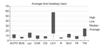
Figure 9. Average time headway in Shilchar for different lead vehicle (Sec)
