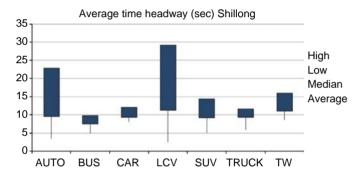
Figure 8. Average time headway in Shillong for different lead vehicle (Sec)
