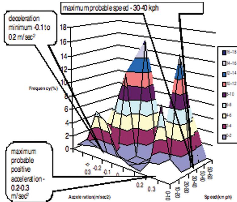
Figure 1 - Speed acceleration frequency joint probability function
