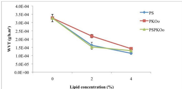
**Fig. 1:** WVT of Chitosan-Lipid Edible Film as a Function of Lipid Concentration (Error Bars are Standard Error of the Mean of Three Measurements).
