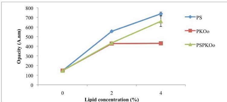
**Fig. 2:** Opacity of Chitosan-Lipid Edible Film as a Function of Lipid Concentration (Error Bars are Standard Error of the Mean of Three Measurements).
