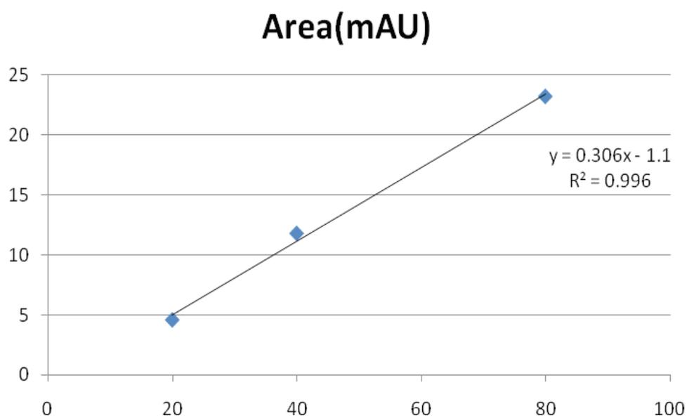
**Figure 5.** Standard calibration plot for caffeine
